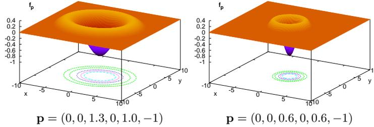
Fig. 5: Proposed regression function  $f_{\mathbf{p}}(\mathbf{x})$  for the approximation of the scale space shapes of the input blobs as shown in Fig. 4. Two examples with different covariance matrix  $\Sigma$  are shown.
