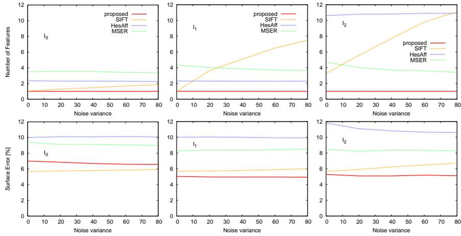
Fig. 7: Comparison of the number of detected features (top row) and the mean *Surface Error* (bottom row) for the three synthetic test features and the four region localization methods. In case of ambiguous detection results, the best is chosen for the *Surface Error*. From left to right: feature types  $I_0$ ,  $I_1$ , and  $I_2$
