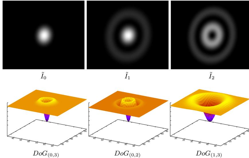
Fig. 4: Resulting image signal  $DoG_{(o,i)}$  of interval  $i$  in octave  $o$  using the scale selection of SIFT. The synthetic test images are shown on top. Each of the input features  $\tilde{I}_0, \tilde{I}_1, \tilde{I}_2$  depict a sinc ( $r$ ) =  $\frac{\sin r}{r}$  shape in the selected scale (bottom).
