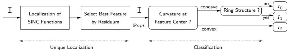
Fig. 6: Workflow diagram of localization and classification of the input image  $I$ .
