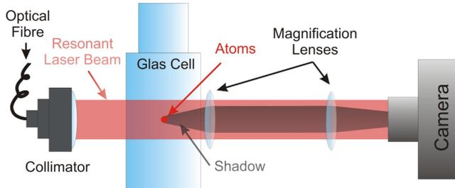
Fig. 1: Simplified sketch of the imaging system. The atomic cloud is illuminated by collimated resonant laser light from an optical fibre. The shadow from the atoms is imaged by a magnifying lens system onto a CCD-Camera. Subtraction from an image without atoms leads to the atomic density distribution.
