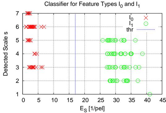
Fig. 8: Energy values  $E_S$  for the real experiment data for the feature types  $I_0$  and  $I_1$  of different sizes. It is shown that a simple threshold value  $thr$  is sufficient to separate the two classes. The classification is independent of the detected scale.
