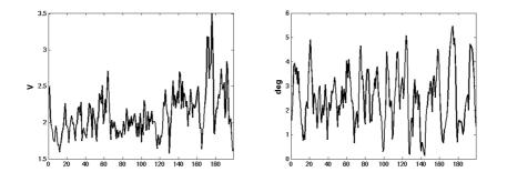
Fig. 13.14. Left: Energy of estimate for walking sequence (200 frames). Right: Error of estimate (left and right knee).
