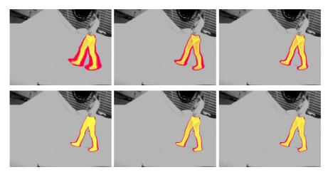
Fig. 13.12. Weighted particles at t = 0, 1, 2, 4, 8, and 14 of *ISA*. Particles with a higher weight are brighter, particles with a lower weight are darker. The particles converge to the pose with the lowest energy as t increases.
