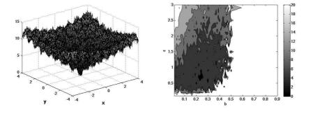
Fig. 13.7. Left: Ackley function distorted by Gaussian noise with standard deviation 0.5. Right: Average time steps needed to find global minimum with error less than  $10^{-2}$  with respect to the parameters *b* and *c*.
