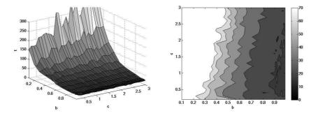
**Fig. 13.5.** Average time steps needed to find global minimum with error less than  $10^{-3}$  with respect to the parameters *b* and *c*.
