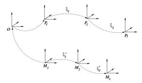
Fig. 13.10. Transformation of rigid body motions from prior data  $P_i$  in a current world coordinate system  $M_1$ . A proper scaling of the twists results in a proper damping.
