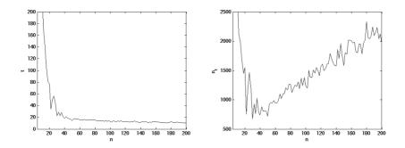
Fig. 13.6. Left: Average time steps needed to find global minimum with respect to number of particles. Right: Computation cost.
