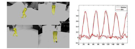
Fig. 13.11. Left: Results for a walking sequence captured by four cameras (200 frames). Right: The joint angles of the right and left knee in comparison with a marker based system.
