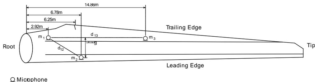
Figure 2. Principle drawing of the rotor blade and microphone positions.
